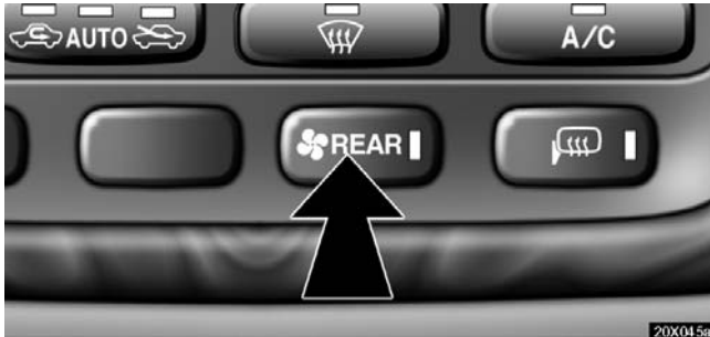
(c) Rear air conditioning switch
