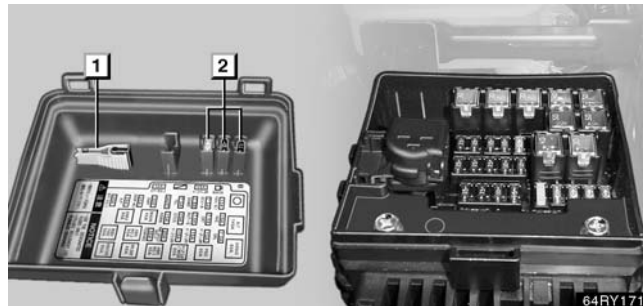
► Engine compartment [1] Pull-out tool [2] Spare fuses
