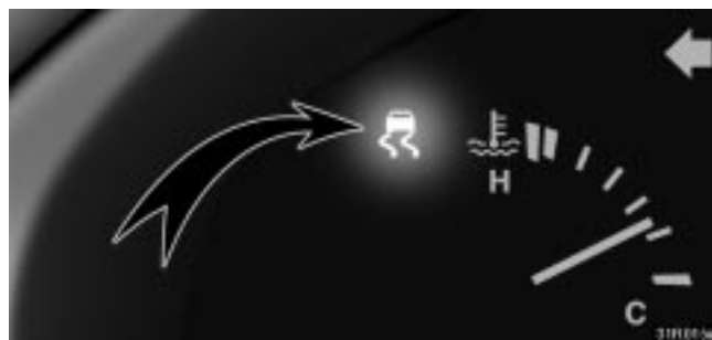
► Slip indicator light
