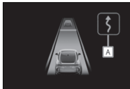
A Curve speed reduction control display
