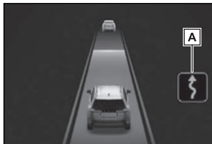
A Curve speed reduction control display
